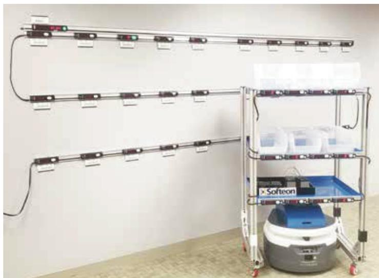
*Image of Softeon Warehouse of the Future Innovation Lab showing pick-to-light technology and mobile robot from Fetch Robotics*
